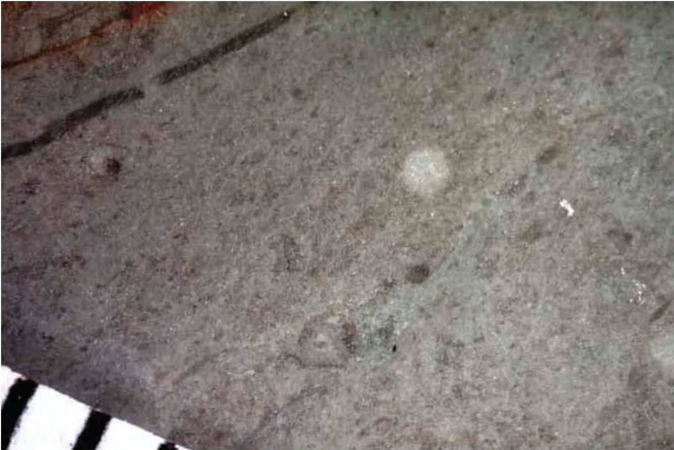
Figure 6. Cherty limestone (scale is marked in millimeters).
