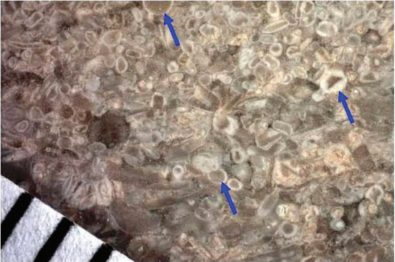
Figure 5. Packstone (scale is marked in millimeters).
